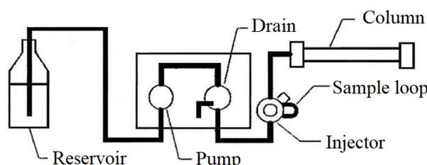
★ **Mix the mobile phase in advance and flow with a single pump. Never mix solvents in a HPLC instrument.**
